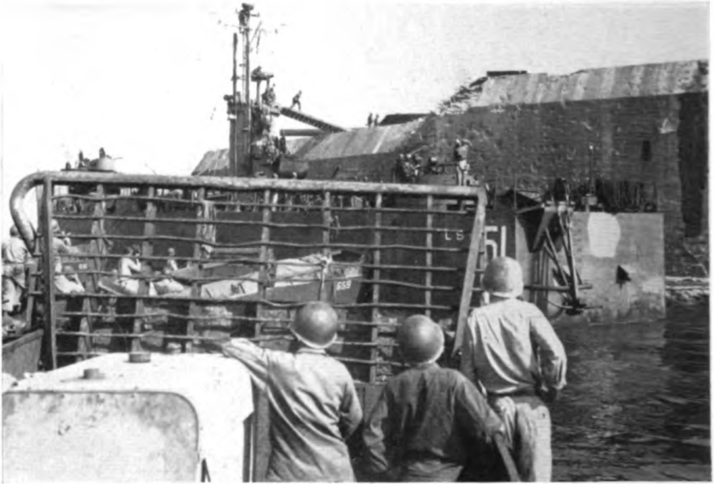
Engineers landing on Fort Drum (El Fraile Island) in Manila Harbor by special ramp from the bridge of an LSM to the top of the fort wall. The LSM is from the Seventh Amphibious Fleet; LCVPs and the LCM are from the 2d ESB. (Signal Corps photo)
